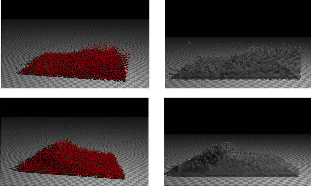
**Figure 5:** The example implemented in original SPH [MCG] method with 8000 large particles.
